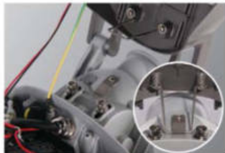
When maintaining LED light, upper cover with support bar which is easy and convenient
